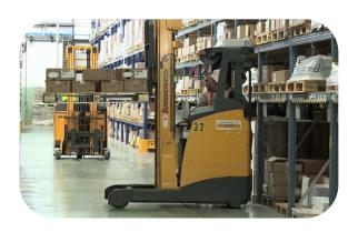
SafeTrack, Essensium's Collision Avoidance Assistance System proves effectively to enable more than just detecting potential Collisions. By knowing what, and where something is, it can populate the WMS or allow more efficient flow of goods. In addition, the data gathered proves to be a valuable source of information to perform some Business Intelligence exercises, not only limited to safety.
