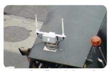
A unique, patented, radio technique gives highly accurate distance measurements even at long range and in the difficult environment of a container terminal. Combined with GPS, a PDS server, and inter-vehicle ranging, this provides multiple levels of redundancy for reliable operation.
